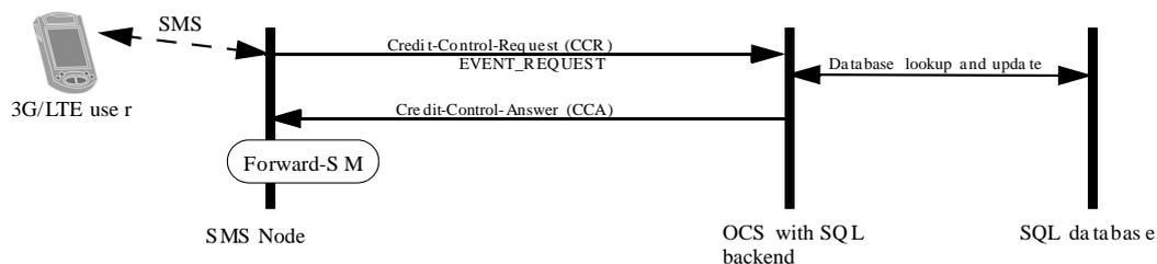
An example of session based online charging using Unit Reservation is shown in Figure 5. Here the user surfs web with prepaid data plan and OCS deducts 3 515 181 bytes from the available data.
